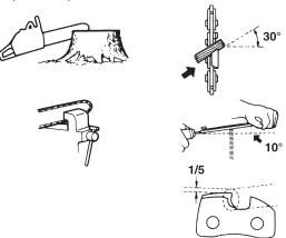
After each cutter has been filed, check the depth gauge and file it to the proper level as illustrated.
